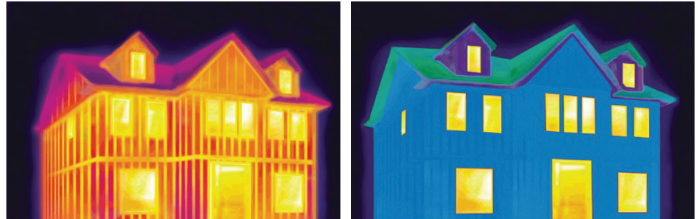
Figure 1. Thermal image illustration of (a) unmitigated thermal bridges with only cavity insulation between framing members and (b) use of ci to minimize thermal bridging. (Similar results can be expected in commercial buildings with and without ci.)
