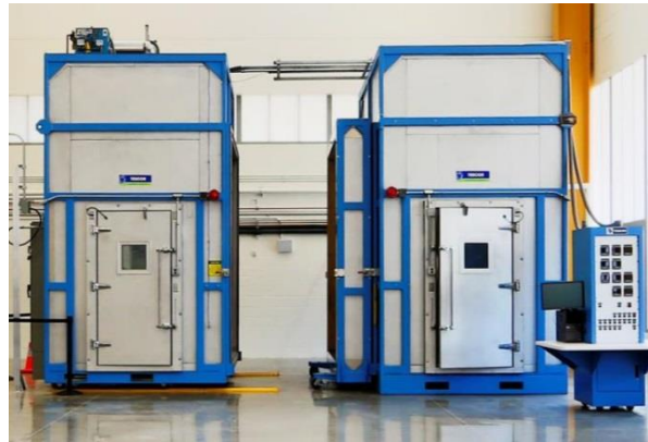
Figure 9. Air and moisture penetration test chamber
