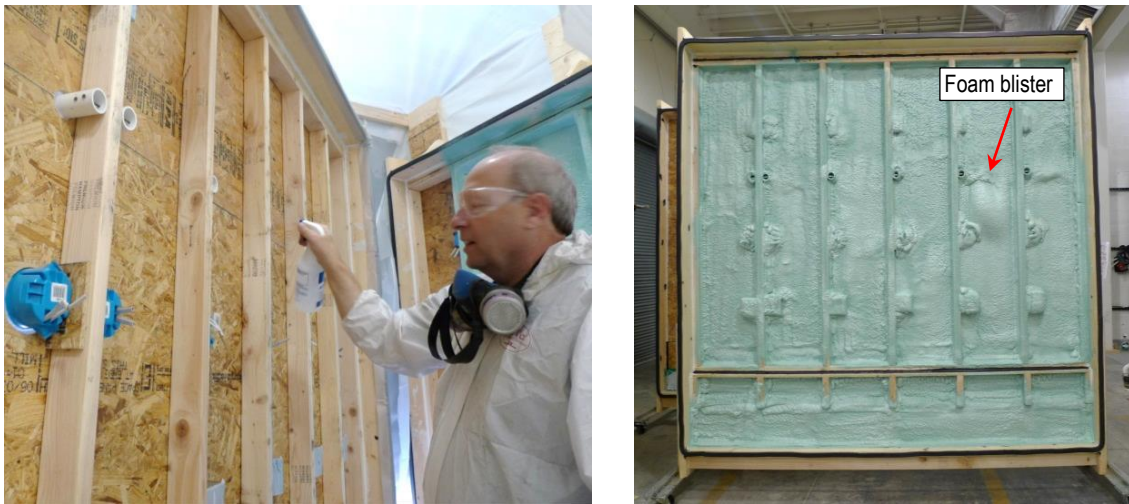
Figure 34. Test wall where 1” closed-cell foam was applied over damp surfaces.
