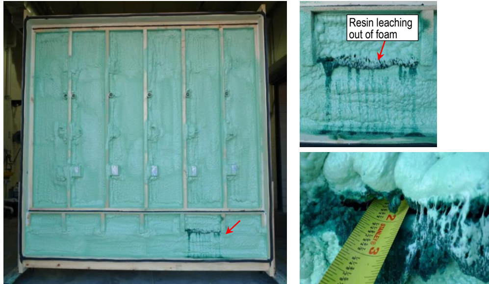
Figure 38. Test wall where a resin-rich foam mixture was utilized.
