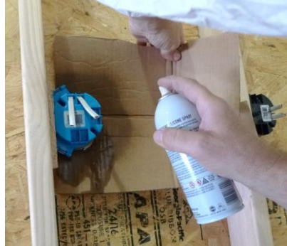
Figure 36. Penetrations sprayed with silicone to simulate an oil film that would compromise the adhesion of the foam to surfaces.
